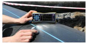
The device implements the Distance Amplitude Correction (DAC) and Time Varied Gain (TVG) functions, with the setting up to 16 points, which allows the operator to evaluate the equivalent reflector size at various depths.
