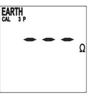
Symbol CAL: indicates that the instrument was calibrated; this symbol is displayed for each subsequent measurement even though the instrument is switched off and on again.
