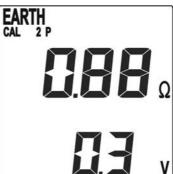
Value measured for earth resistance  $R_A + R_T$
