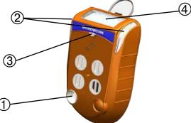
In the alarm state, Gas-Pro will vibrate, its sounder ① will emit a rapid tone, the alarm LEDs ② will flash red and blue, the +ve Safety™ indicator ③ will be off in alarm, the LCD display ④ will also be red and highlight the gas in alarm.
