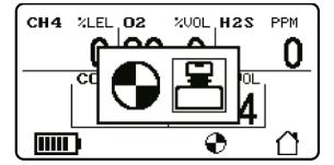
Click the operator button to highlight for Pump or for Bump testing and then double click to select (see *Pump test* on *page 20* or *Speedy bump* on *page 41* and *Smart bump* on *page 41* for Bump details).
