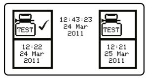
The next screen indicates when the Gas-Pro was last calibrated. It also indicates when the next calibration is due with a warning symbol next to the number of days left, if this is fewer than 30 days. If the calibration due date has expired, the number of days figure is not displayed and the warning symbol flashes.
