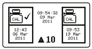
If the calibration due lockout feature has been enabled the lockout icon **(iii)** will be displayed and the Gas-Pro will not proceed past this point.
