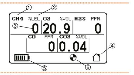
In 'clean air',  $CO_2$  and Oxygen levels are typically 0.04% and 20.9% respectively. In zero mode, these gases will actually run an 'offset' zero.
