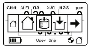
Upon entry to Tank Check Mode, the device will display a confirmation message to inform that alarms are disabled. A single button press will dismiss this screen. The confirmation screen is accompanied by an intermittent warning tone.
