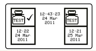
Gas-Pro will not inform the user of a need for a gas test until the interval period from the last successful bump has expired. However on applying a magnetised flow plate, or placing Gas-Pro into the Q-Test the user will be given the option to complete a gas test (or proceed to pumped operation).
