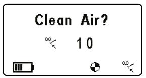
An Autozero should not be performed unless the Gas-Pro is in clean air. Press the operator button to enter the Autozero mode, otherwise the countdown will progress and will not perform a zero.
