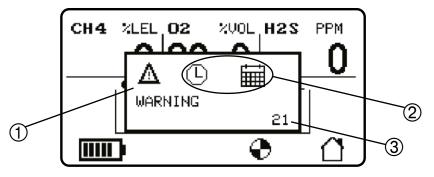
The warning triangle ① indicates faults that can be rectified by the user. The symbol is accompanied by the text "WARNING" below. The warning triangle is replaced by a spanner and screwdriver for faults which require service and the text "SERVICE" below. For the low battery warning the "WARNING" text is replaced by "ALERT".
