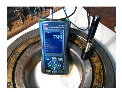
Device can be equipped with different types (D, DC, DL, C, D+15, E, G) of Leeb probe. Standard set of the device is included D type (universal) Leeb probe, other types by request.
