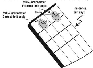
Fig. 7: Positioning the inclinometer M304
