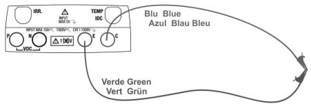
Fig. 13: Compensation of the measuring cables' resistance
