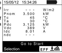
13. Keeping the remote unit SOLAR-02 always close to the main unit, press the **GO/STOP** key on PVCHECKS to start testing. The message "**Waiting start recording...**" appears on the display of the main unit and "**HOLD**" is shown on the display of SOLAR-02, together with an indication of the time remaining, expressed in seconds, until "00" is reached.
