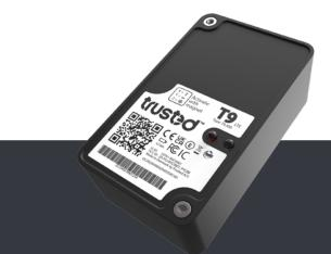
**T9LTE** is a small IoT tracking device and data logger that offers **asset monitoring and data tracking** of any asset; from non-powered equipment to entire fleets.
