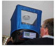
By simply adding the 400 mm x 400 mm short canvas (as illustrated), a starting volume of 5 l/sec, 18 m<sup>3</sup>/hr, 11 cfm is achievable and being only 610 mm high, it gives easy access to the grills.
